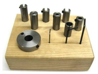
I make bases out of maple to hold this adapter, bushing and cutter in whatever orientation is needed. The one I use to make and sharpen each of the boring bar cutter's edges is shown here. Such bases can be made for
