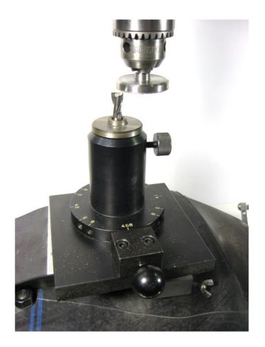
The idea for these bases came originally from an end mill sharpening jig I bought. The diamond wheel is especially good for end mills because it holds the perfectly crisp edge needed to get right up to the center cutting gash. Unfortunately, the purchesed jig will only do the primary end angle and not the secondary or gash angles. But even doing just the primary angle a few times dramatically reduces the cost of end milling.
