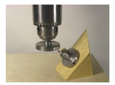
bars which take custom cutters in three different sizes. These could be a nightmare to make and maintain without a jig. To hold them, I made this simple adapter and set of bushings to accommodate 1/8", 3/16" and 1/4" HSS round and square tool bits.
